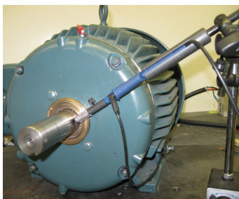
Figure 4. Testing of 10HP motor with CMCs.
